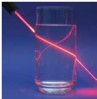
Figure 3.21 This beam of red light allows you to see the path of light bend as it enters and leaves the water.
